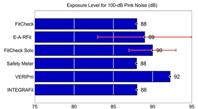
Figure 2. Estimated A-weighted Exposure Levels for six fit-test systems.
