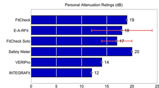
Figure 1. Personal Attenuation Ratings for six fit-test systems.
