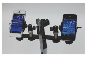
Figure 1. The SoundMeter app on the iPhone 5 (left) and iPhone 4S (right) compared to <sup>1</sup>/<sub>2</sub>" Larson-Davis 2559 random incidence type 1 microphone (center).
