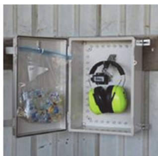
Figure 3. Hinged weatherproof aluminum box containing HPDs
