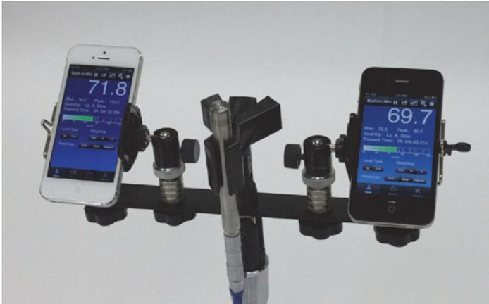
Figure 1. The SoundMeter app on the iPhone 5 (left) and iPhone 4S (right) compared to 1/2" Larson-Davis 2559 random incidence type 1 microphone (center).
